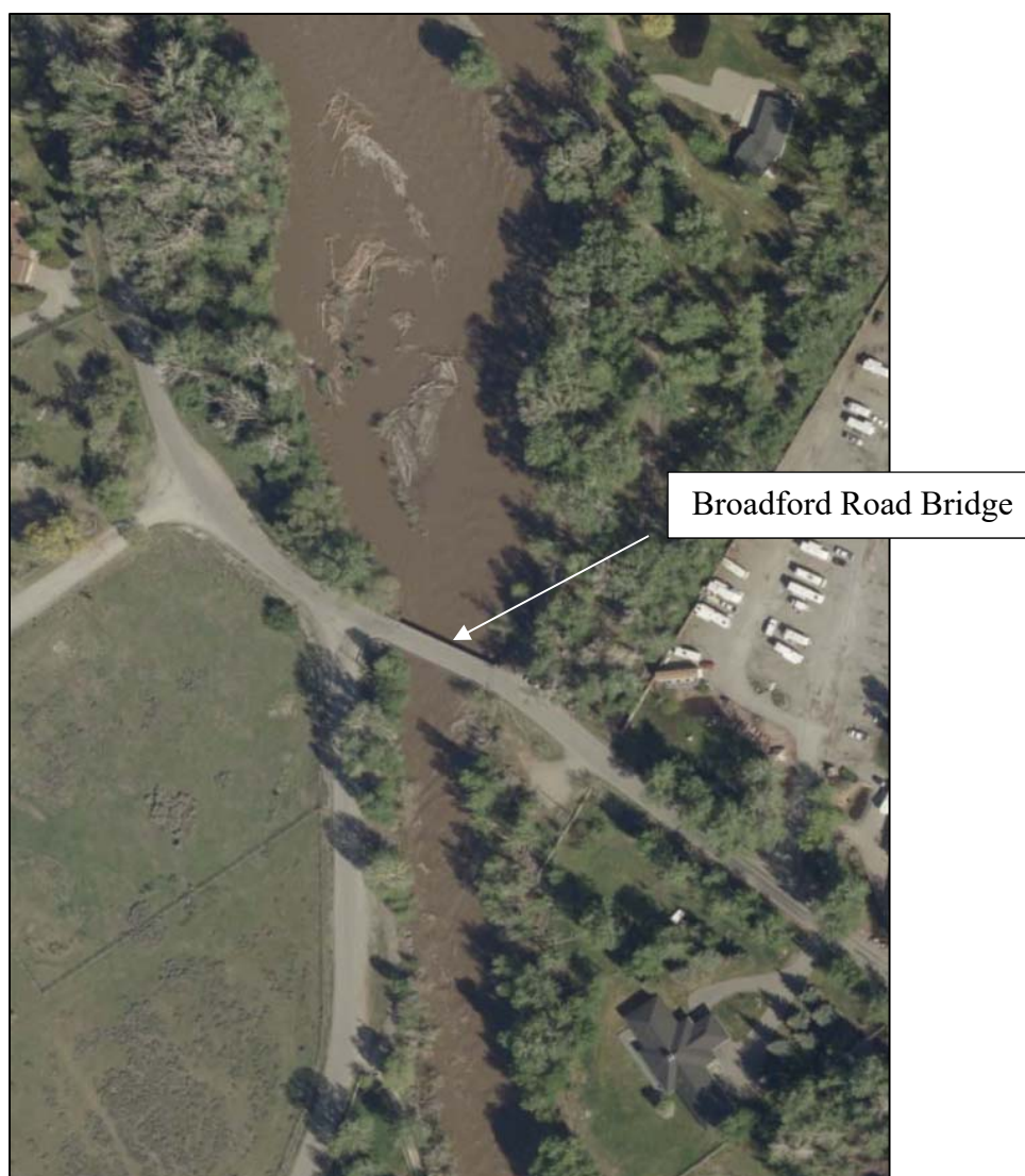
Figure 4. The narrow span of the Broadford Road Bridge restricts floodplain conveyance and maintains a bottleneck that constricts debris, sediment, and flood water conveyance.
